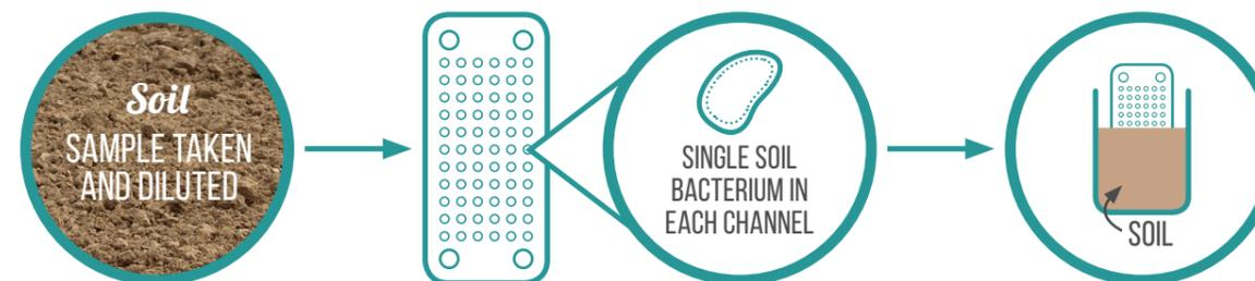
A DEVICE REFERRED TO BY RESEARCHERS AS THE 'iCHIP' WAS USED TO CULTURE SOIL BACTERIA ALLOWING NUTRIENTS & SIGNAL MOLECULES TO PASS TO THE BACTERIA & STIMULATE GROWTH.
