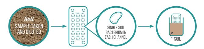
A DEVICE REFERRED TO BY RESEARCHERS AS THE 'ICHIP' WAS USED TO CULTURE SOIL BACTERIA ALLOWING NUTRIENTS & SIGNAL MOLECULES TO PASS TO THE BACTERIA & STIMULATE GROWTH.
