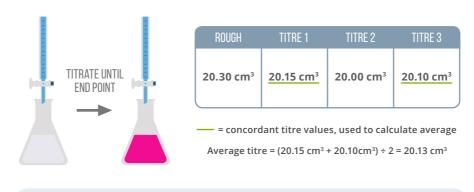
To carry out the titration, the tap of the burette is opened to allow the solution inside to flow into a known volume of the solution in the conical flask. The amount of solution from the burette required to reach the end point is recorded. A rough titration is usually followed by more accurate runs. Multiple titrations are carried out until concordant titres are obtained (within 0.10 cm³ of each other).
