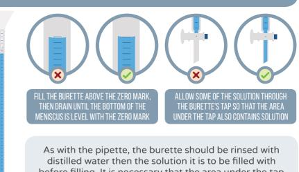
As with the pipette, the burette should be rinsed with distilled water then the solution it is to be filled with before filling. It is necessary that the area under the tap also contains solution as the burette's scale includes this volume. Without doing this, the volume recorded for titrations would be higher than the actual value.
