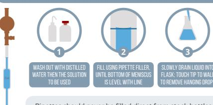
Pipettes should never be filled direct from stock bottles of solution as this could contaminate them. Instead, fill them from some of the solution poured into a beaker. They're calibrated to allow for a small amount of solution remaining in the tip after the correct volume has been delivered, so this remainder shouldn't be forced out.
