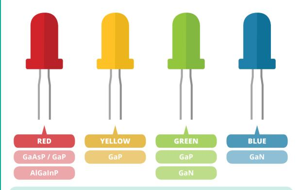
LEDs (light-emitting diodes) give off light when current is passed through them. They are made from semiconducting materials; the colour of light emitted depends on the materials used. Many of these materials are based on gallium, such as gallium arsenide phosphide (GaAsP), gallium phosphide (GaP), gallium nitride (GaN), and aluminium gallium indium phosphide (AlGaInP).
