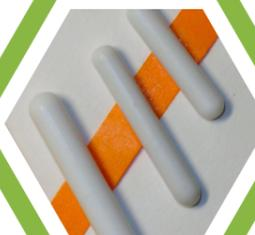
The magnetic stir bars used in many chemical laboratories are coated in an inert polymer (PTFE) which should stop them affecting reactions. However, new research shows that scratches and cracks could track metal particles, which could then interfere with reactions.
