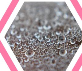
A copper catalyst with structures inspired by a diving bell spider's air-trapping hairs helps conversion of carbon dioxide from the atmosphere into useful chemicals. The structures increase the CO<sub>2</sub> concentration near the catalyst and reduce the formation of hydrogen gas waste.
