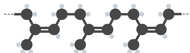
SECTION OF NATURAL RUBBER'S REPEATING STRUCTURE
